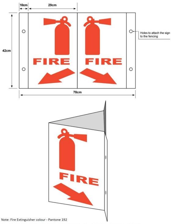
The sign should be fixed to the fence, facing the track, at least 2 metres above the track level.
